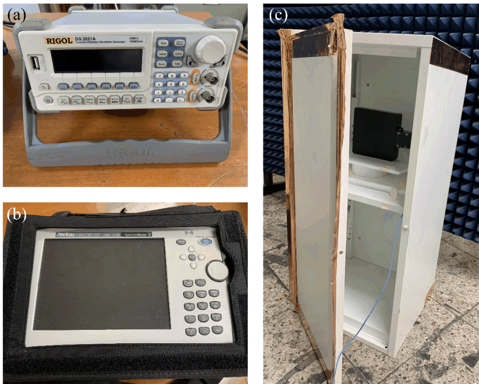
Figure 7. SE measurement setup: (a) function generator; (b) spectrum analyzer; and (c) loop antenna within the commercial metallic cabinet.
